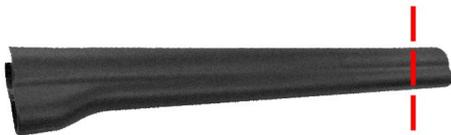
6. Snap the cover around the turn signal wires and the steering column. Secure any loose wires behind the dash.
